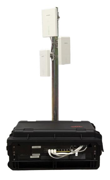
The OBE 5G Flyaway brings professional broadcast encoding to the bonded cellular market. Tier 1 sports broadcasts can now be transmitted over 5G at high bitrates with strict MPEG-TS compliance for interoperability, 4:2:2 10-bit video and 16-channel audio. It contains powerful external antennas that can be mounted at height using Power-over-Ethernet to reach as many cell towers as possible. In addition, fibre and satellite internet (e.g Starlink/OneWeb) can be bonded for maximum assurance.
